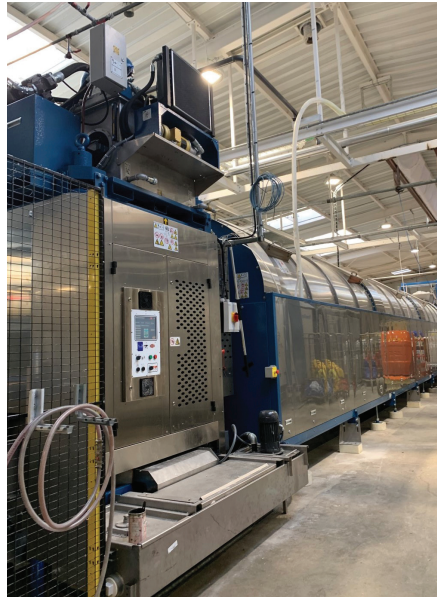
SINGLE STAGE: The new equipment includes an MP1640 single stage press
