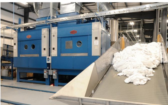
FAST EXTRACTION: Pass-through dryers receive the goods via a loose goods shuttle. The chute lifts up and M-Series tilts 21 degrees forward to discharge linen
