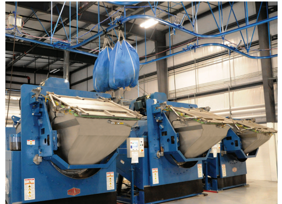
TILT AND SHOOT: The automated chute is also the door, saving time in the loading process ALL IN: The integrated automatic overhead chute-loading door
