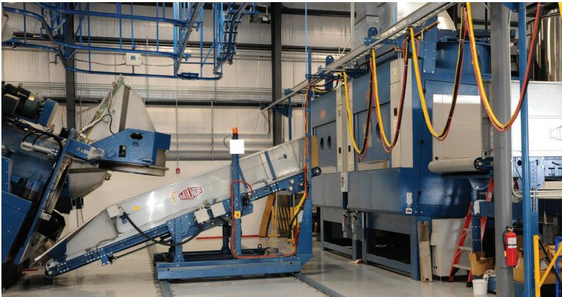
TILT AND SHOOT: The automated chute is also the door, saving time in the loading process ALL IN: The integrated automatic overhead chute-loading door
