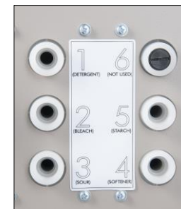
Safe chemical injection
