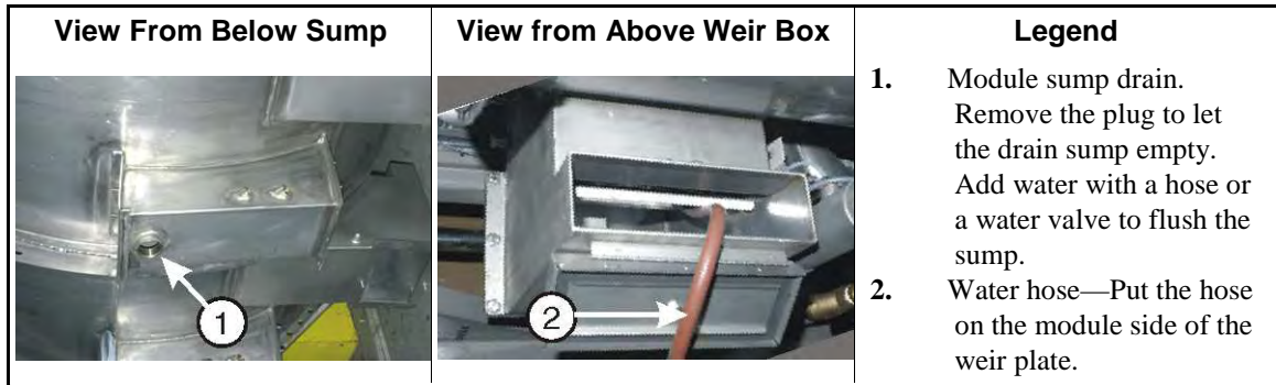
Figure 21: Module Sump Drain and Weir Box. These are examples. Your machine can look different.
