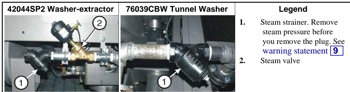
Figure 8: Steam Inlet Strainer. These are examples. Your machine can look different.
