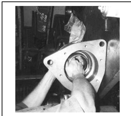
FIGURE 6 (MSSM0303AE) Installing Seal Sleeve in Bearing Housing
