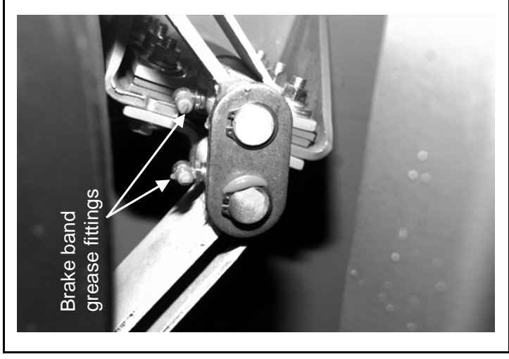
FIGURE 22 (MSSM0201CE) Brake Band Grease Fittings (60044 and 72044WP2/WP3)
