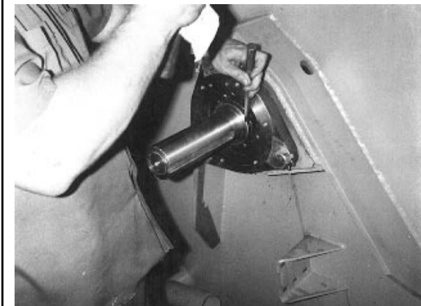
FIGURE 11 (MSSM0303AE) Tightening the Bearing Locknut (42" machine shown)
