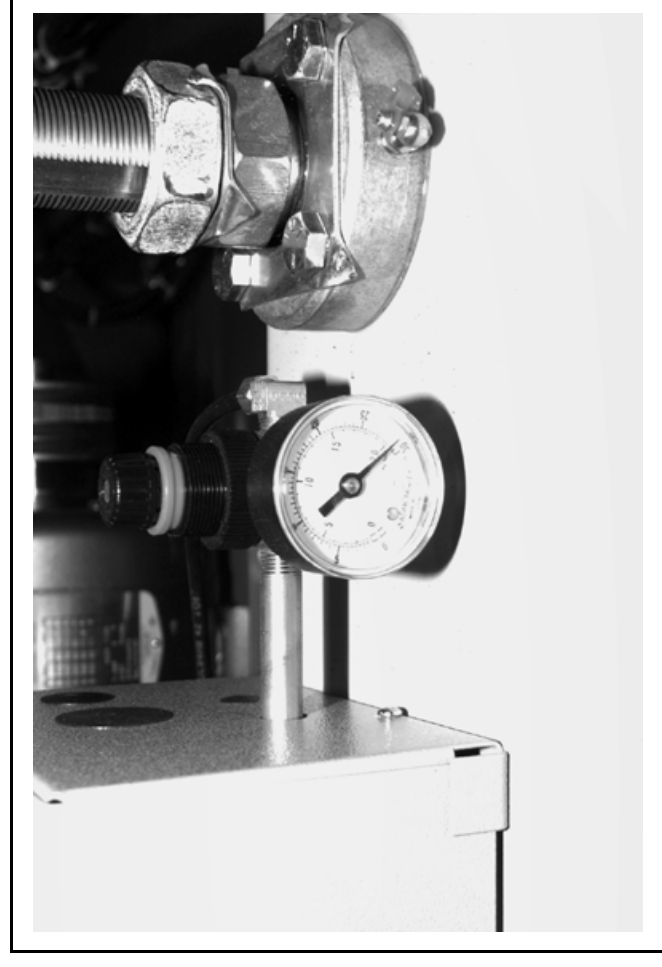
FIGURE 26 (MSSM0201CE) Door Seal Pressure Regulator
