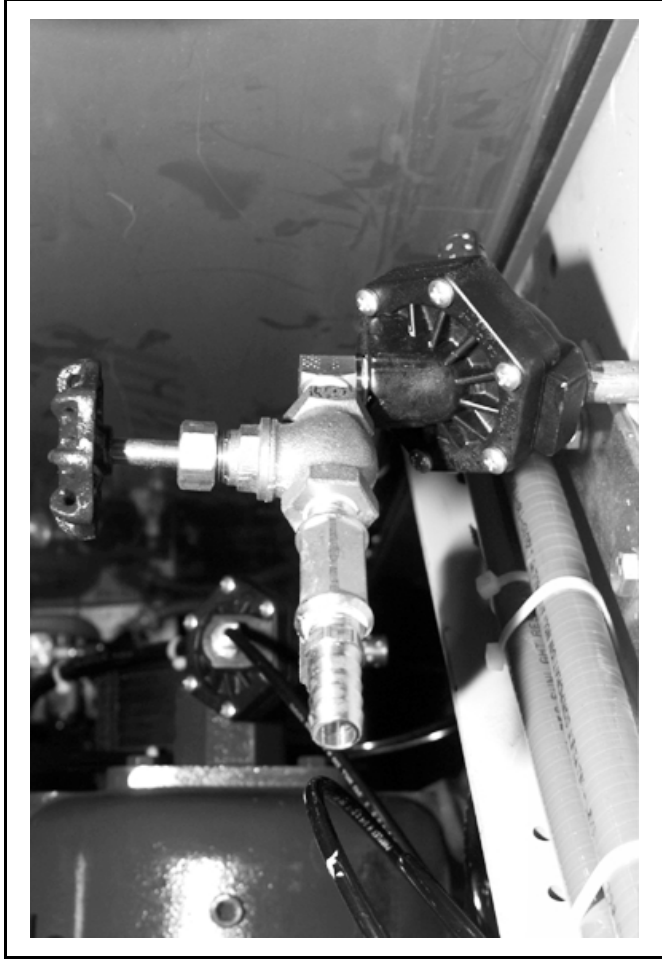
FIGURE 29 (MSSM0201CE) Push-Down Control Valve (72" Rapid load and Staph-Guard® only)
