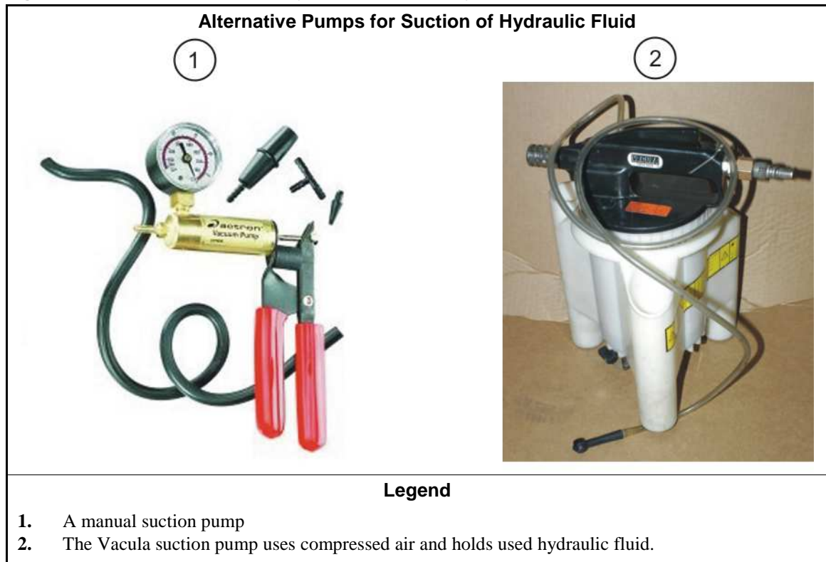
Figure 3: Pumps Used to Remove Hydraulic Fluid Quickly
