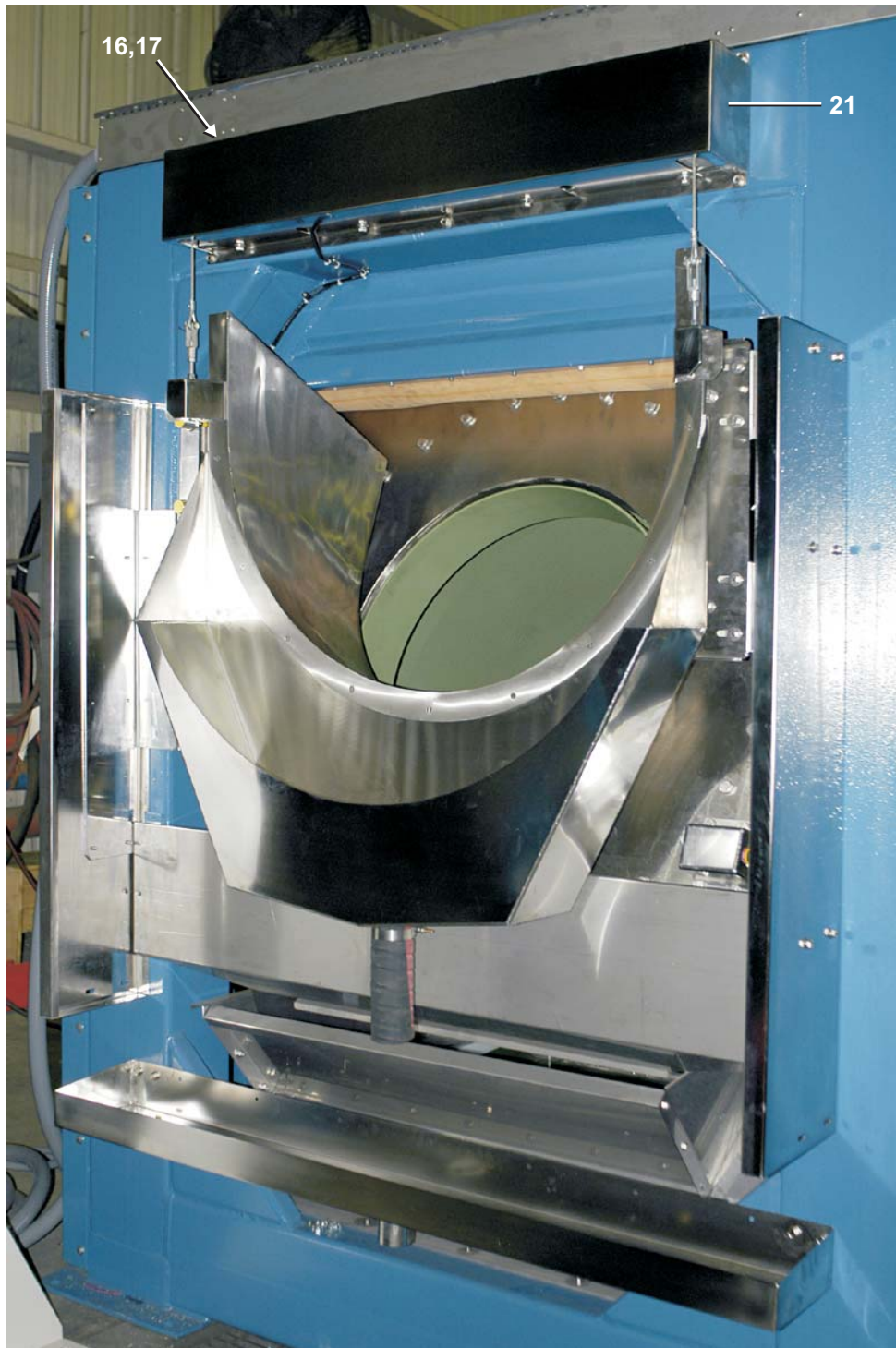
Figure 1: Load Chute Installed
