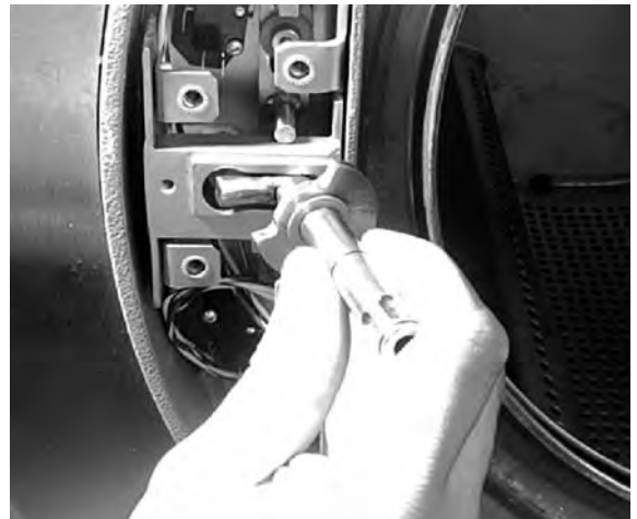
Figure 7: Removing the Shaft from the Lock Mechanism
