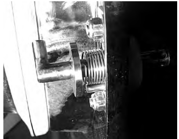
Figure 9: Shaft with Return Spring Installed
