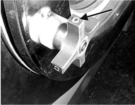
Figure 1: Door Handle Spoke Set Screw
