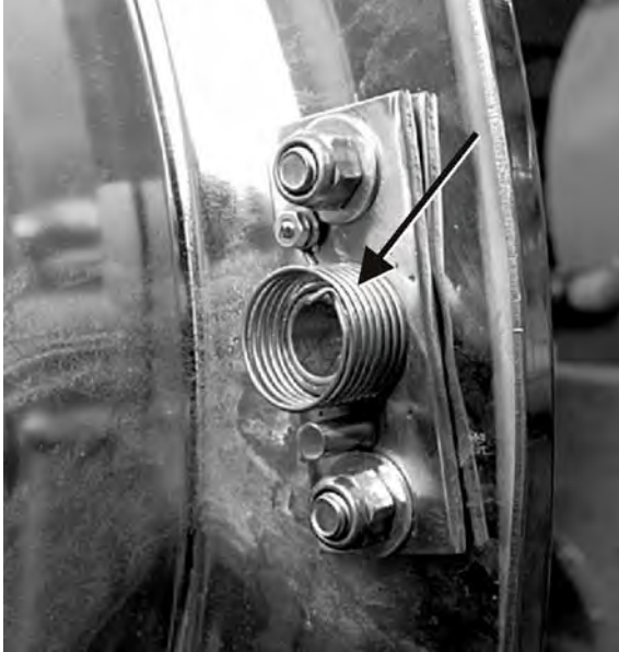
Figure 5: Return Spring After Separation from Shaft Cam
