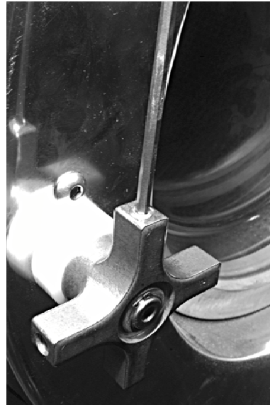
Figure 11: Adjusting Set Screw
