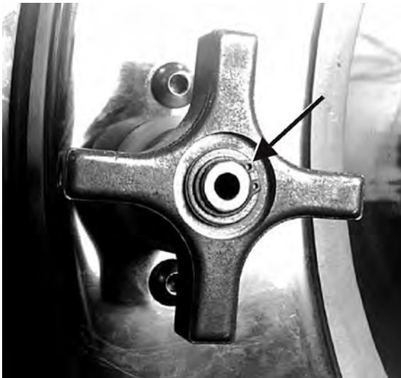
Figure 3: Front Retaining Clip and Thrust Washer
