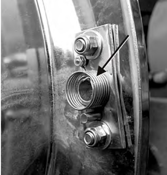
Figure 5: Return Spring After Separation from Shaft Cam
