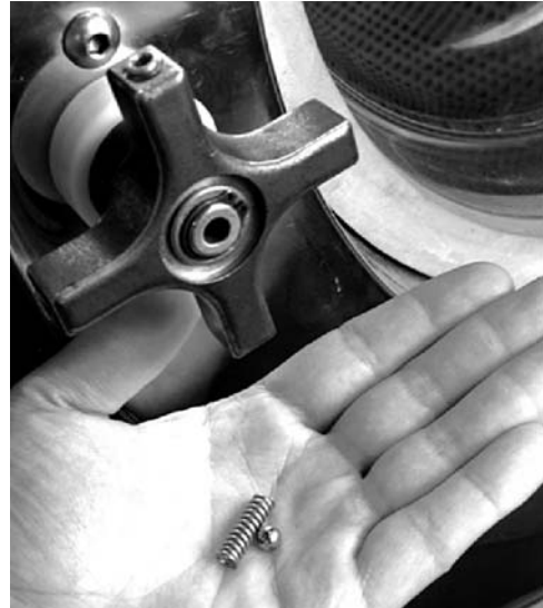
Figure 2: Handle Spoke Spring and Ball
