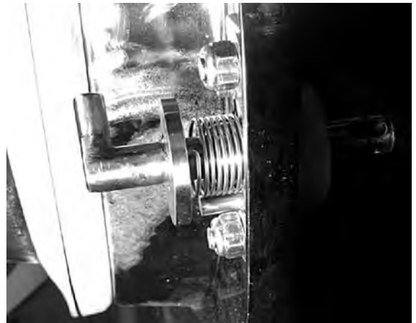
Figure 9: Shaft with Return Spring Installed
