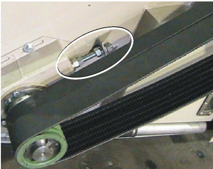
Figure 8. Some Pairs of Tension Mechanisms that Can Change the Angle of the Pulleys
