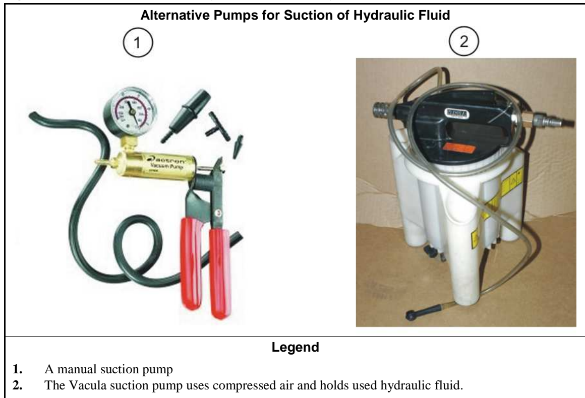
Figure 3: Pumps Used to Remove Hydraulic Fluid Quickly
