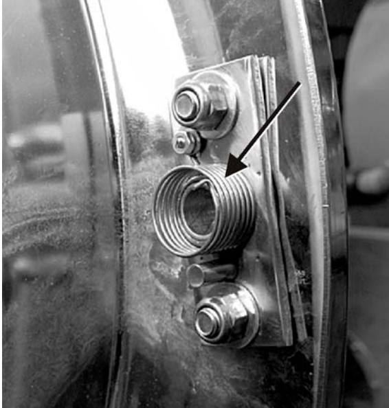
Figure 5: Return Spring After Separation from Shaft Cam
