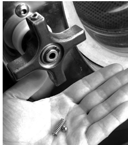
Figure 18. Handle Spoke Spring and Ball
