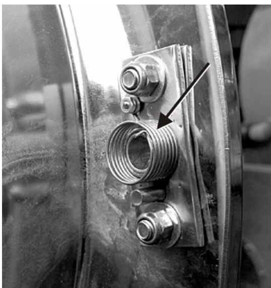
Figure 21. Return Spring After Separation from Shaft Cam
