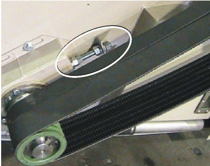
Figure 36. Some Pairs of Tension Mechanisms that Can Change the Angle of the Pulleys
