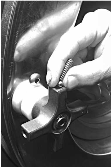
Figure 26. Inserting Ball and Spring in Handle Spoke
