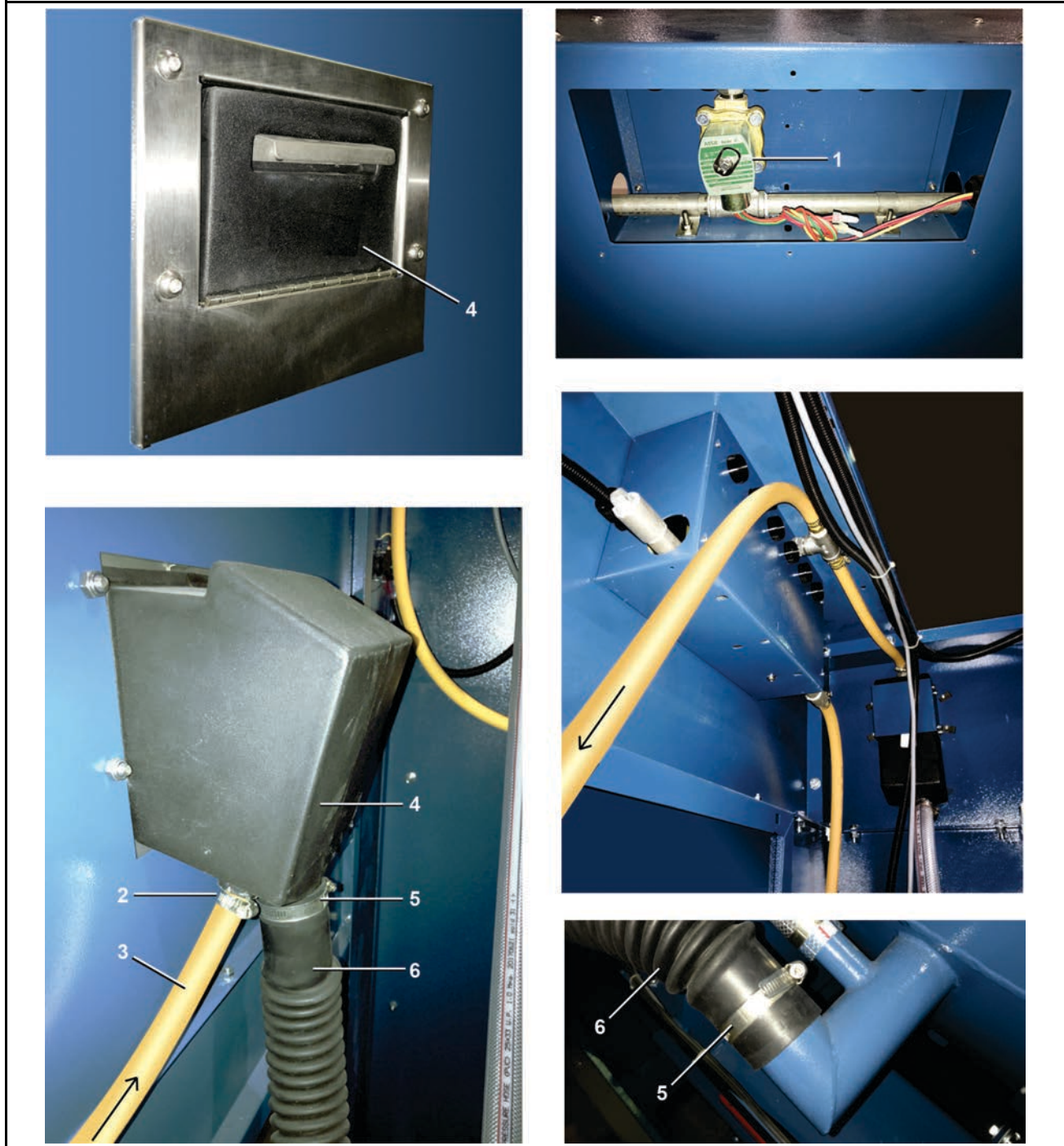
Figure 22. Soap Chute Components and Installation
