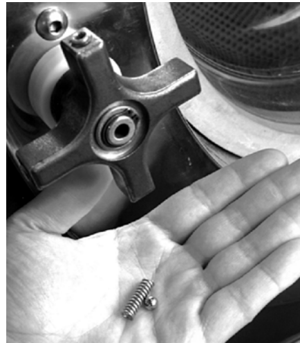
Figure 11. Handle Spoke Spring and Ball
