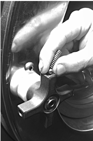
Figure 19. Inserting Ball and Spring in Handle Spoke
