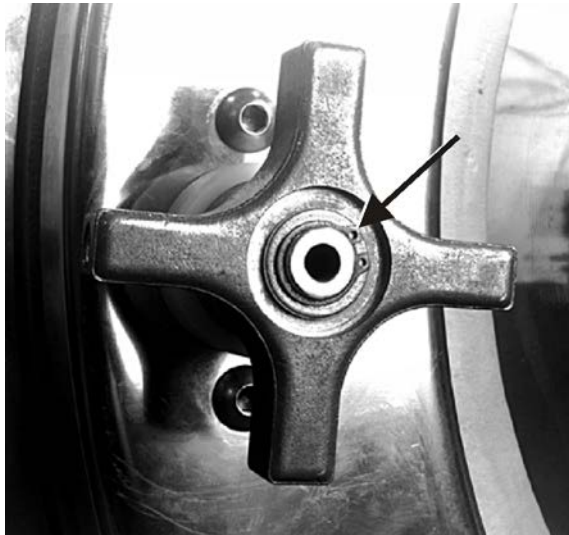
Figure 12. Front Retaining Clip and Thrust Washer
