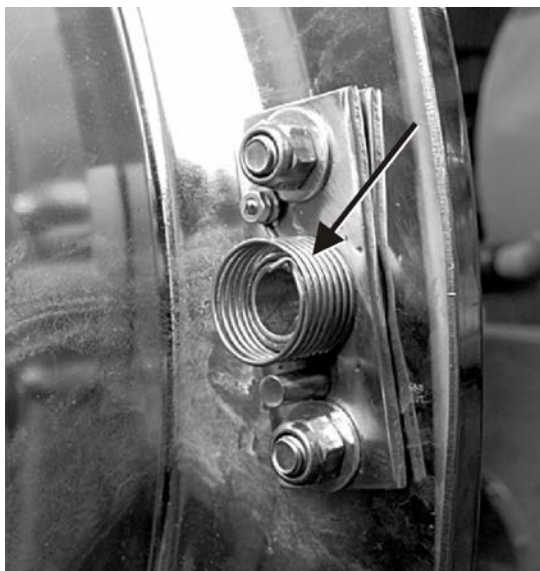
Figure 14. Return Spring After Separation from Shaft Cam
