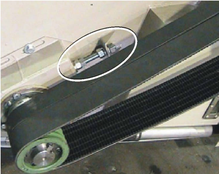
Figure 26. Some Pairs of Tension Mechanisms that Can Change the Angle of the Pulleys
