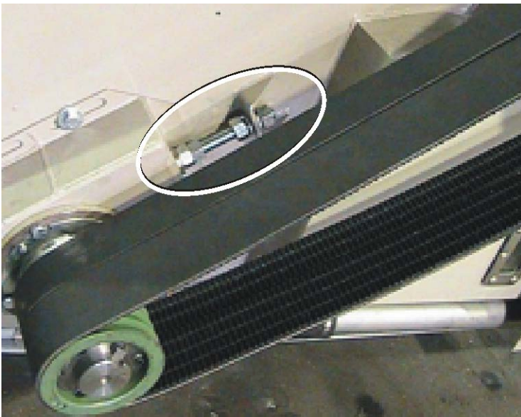
Figure 32. Some Pairs of Tension Mechanisms that Can Change the Angle of the Pulleys
