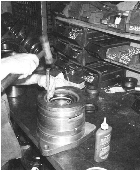
Figure 33. Installing Seals in Bearing Housing
