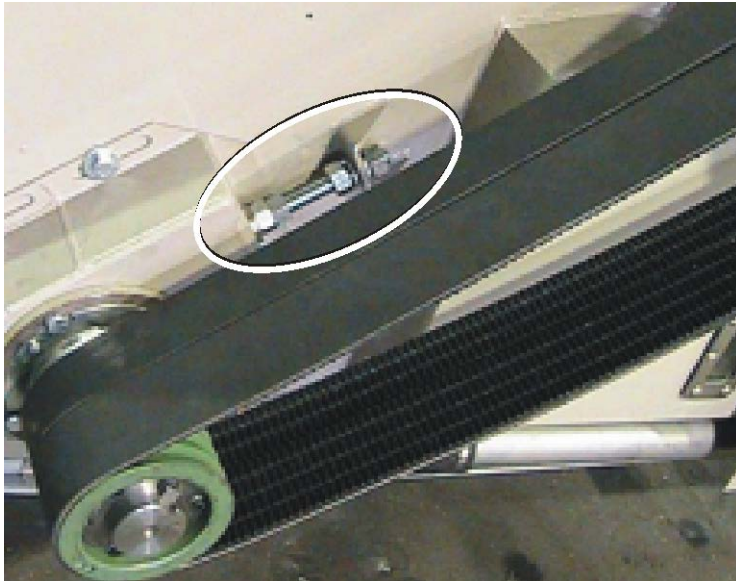
Figure 14. Some Pairs of Tension Mechanisms that Can Change the Angle of the Pulleys
