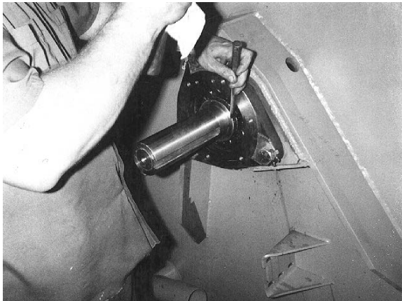
Figure 39. Tightening the Bearing Lock nut (42" machine shown)
