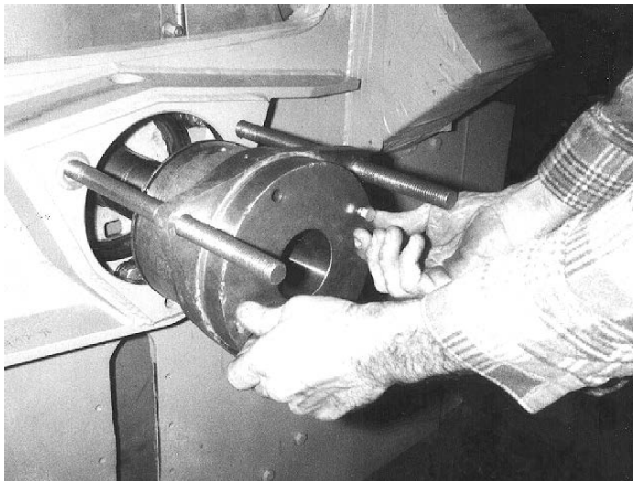
Figure 35. Installing the Bearing Housing Setting Fixture onto Housing (42" machine shown)
