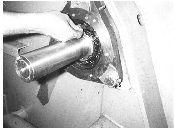
Figure 40. Measuring the Mounted Internal Clearance of the Bearing (42" machine shown)
