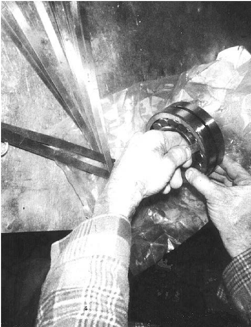
Figure 40. Measuring Bearing Unmounted Clearance (bridge for 42" machine shown)
