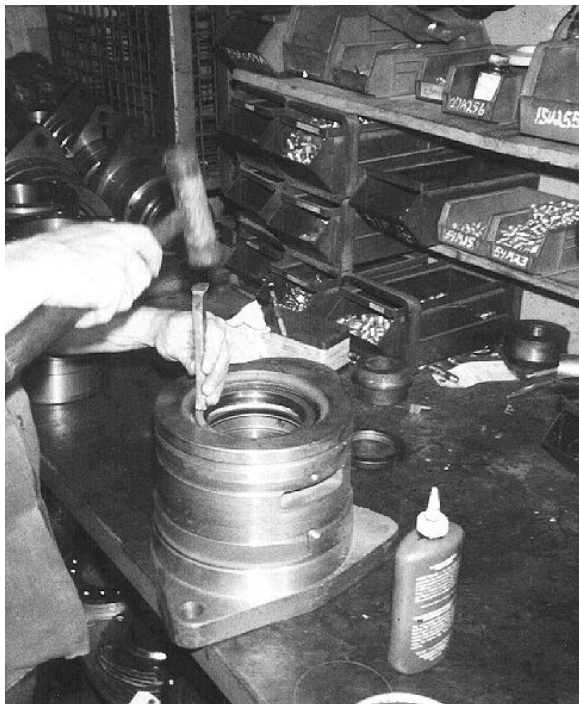
Figure 35. Installing Seals in Bearing Housing
