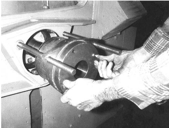
Figure 37. Installing the Bearing Housing Setting Fixture onto Housing (42" machine shown)
