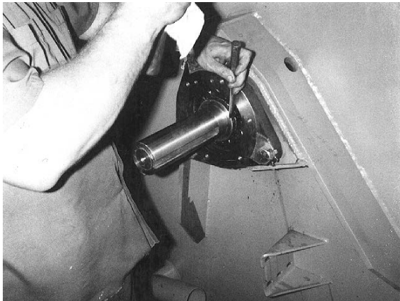
Figure 41. Tightening the Bearing Lock nut (42" machine shown)
