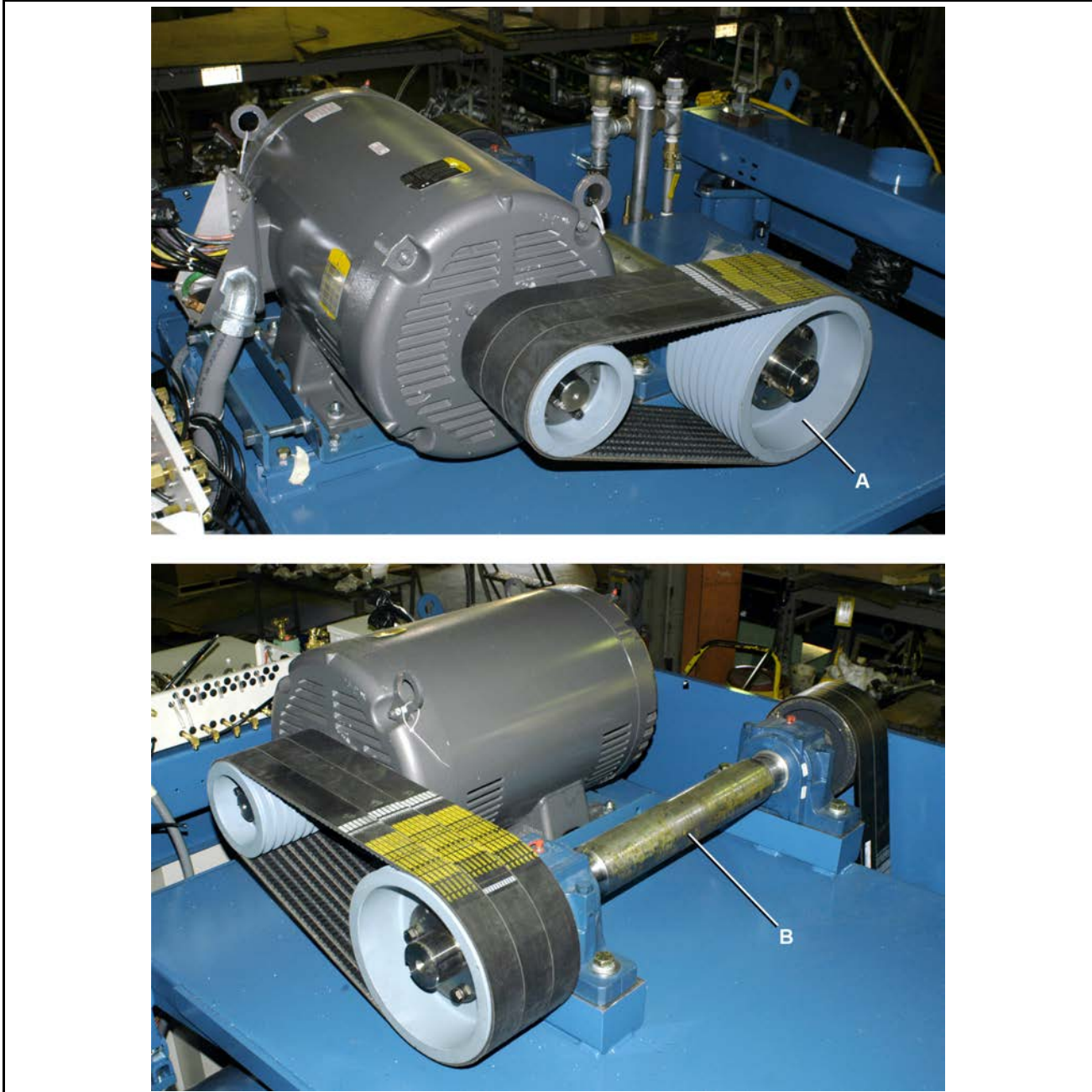
Figure 22. Motor mount, drive shaft, and pillow block bearings
