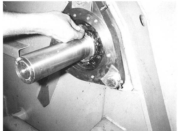
Figure 42. Measuring the Mounted Internal Clearance of the Bearing (42" machine shown)
