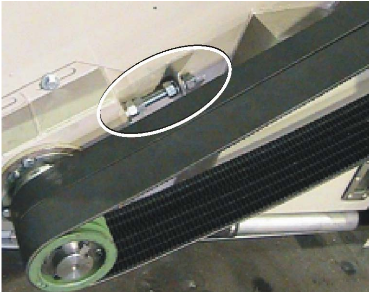
Figure 12. Some Pairs of Tension Mechanisms that Can Change the Angle of the Pulleys
