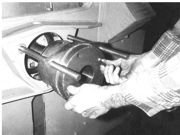
Figure 28. Installing the Bearing Housing Setting Fixture onto Housing (42" machine shown)
