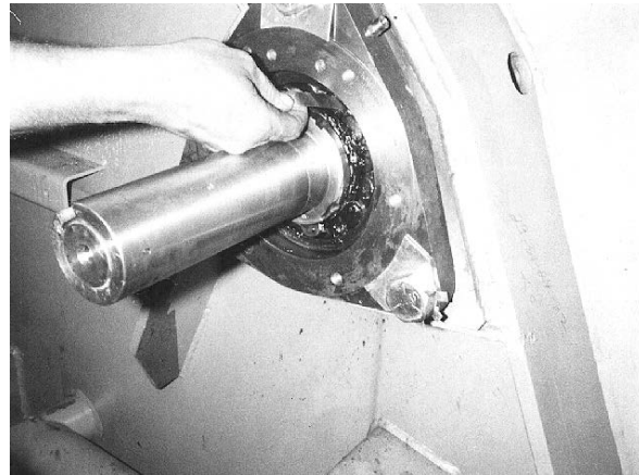
Figure 33. Measuring the Mounted Internal Clearance of the Bearing (42" machine shown)
