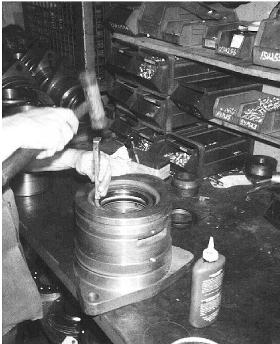
Figure 26. Installing Seals in Bearing Housing
