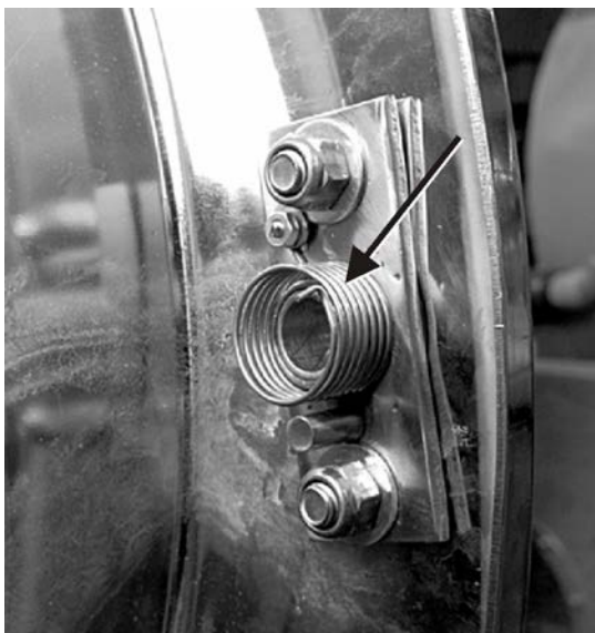
Figure 14. Return Spring After Separation from Shaft Cam
