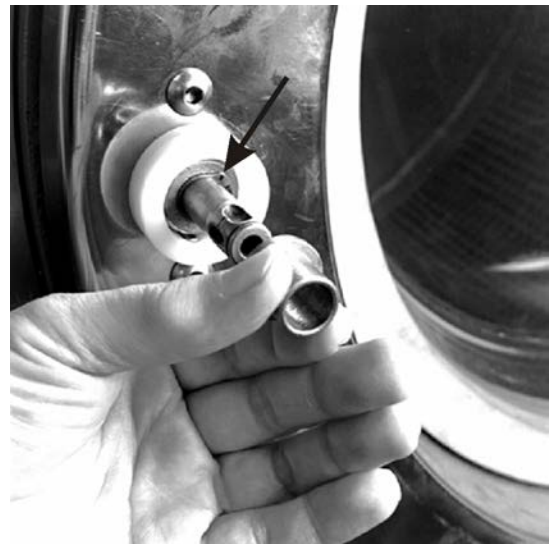
Figure 13. Rear Flange Bearing (being removed) and Retaining Clip (arrow)
