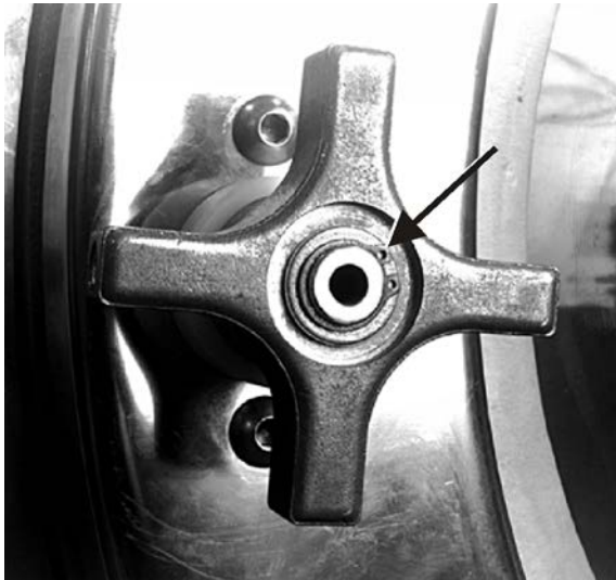
Figure 12. Front Retaining Clip and Thrust Washer
