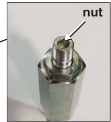
Booster pump relief valve
