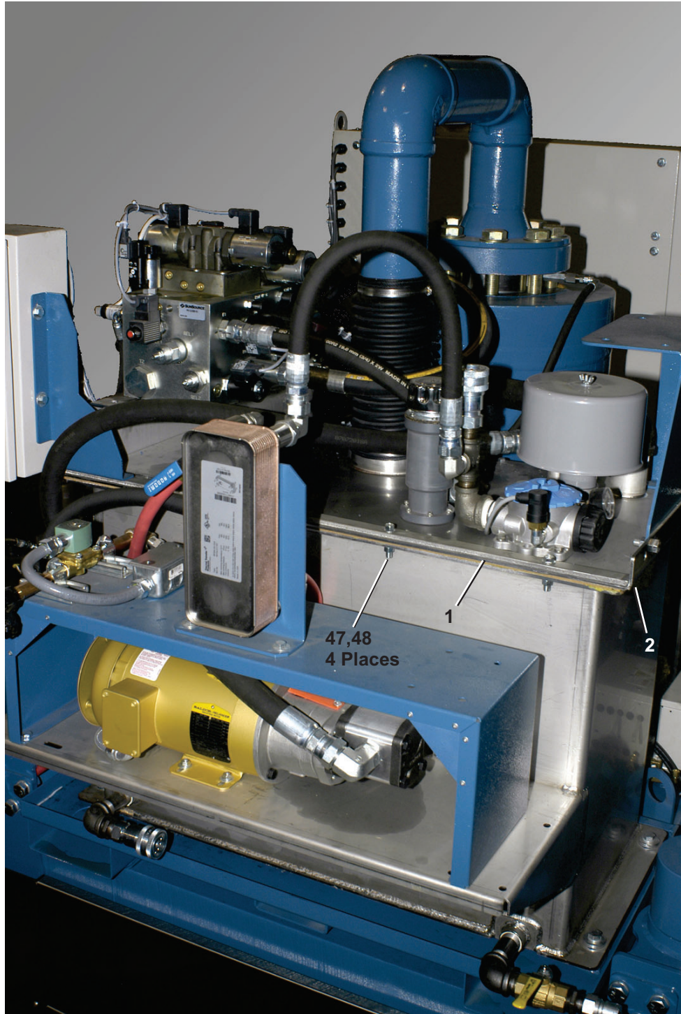
Figure 1: Hydraulic Tank Overview
