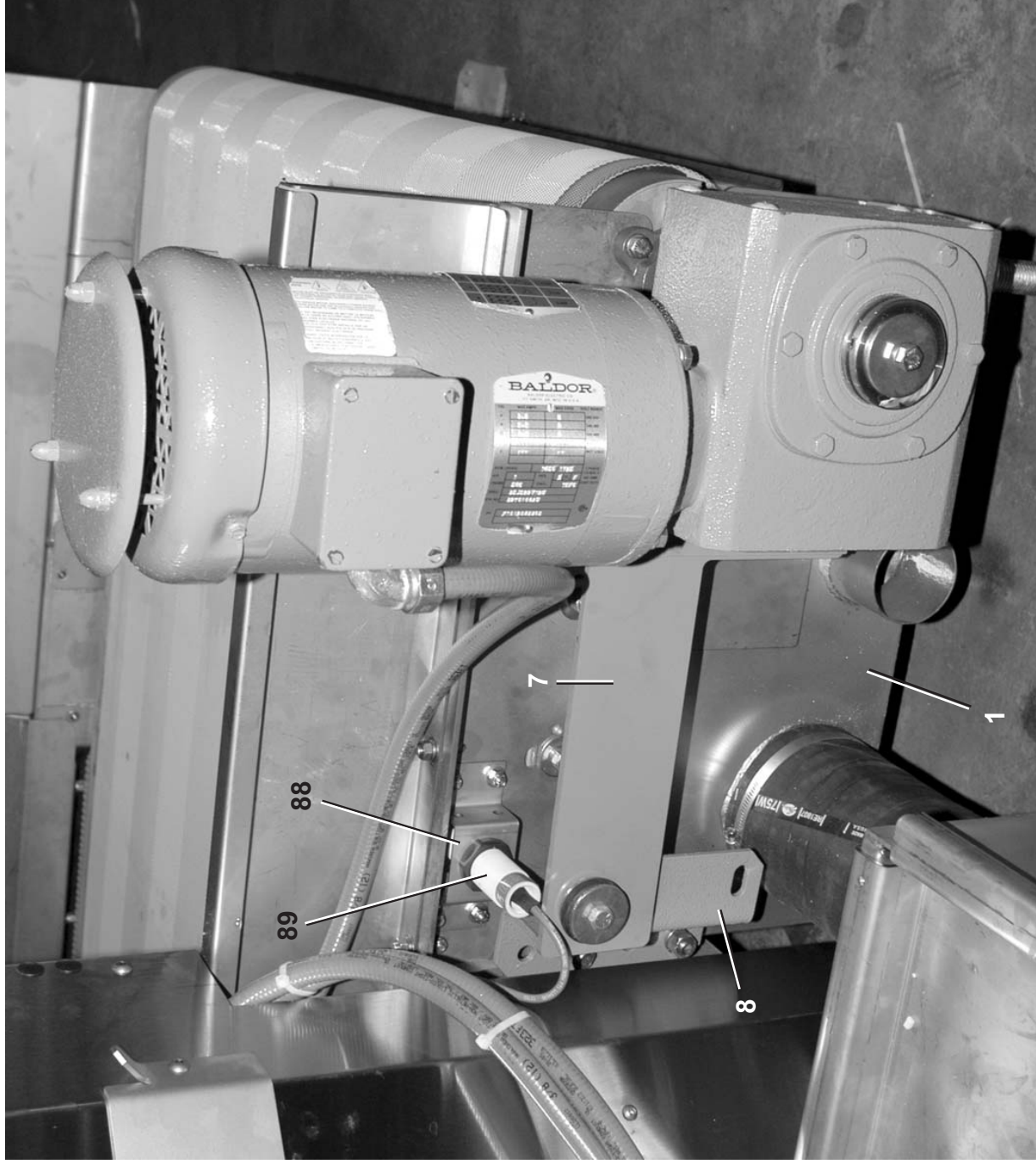
Conveyor Unload End - 0" Bed Extension (00A, 00B)
