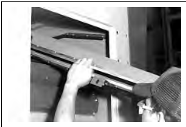
FIGURE 7 (MSSMD447AE) Folding Screen for Removal
