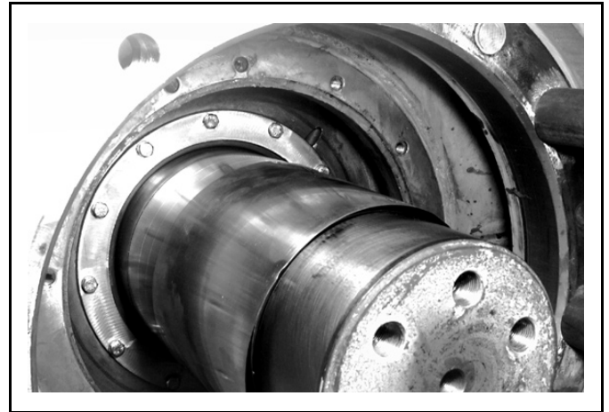
FIGURE 16 (MSSM0275AE) Shim Stock Covering Edge of Shaft Sleeve (Slinger ring removed for clarity)
