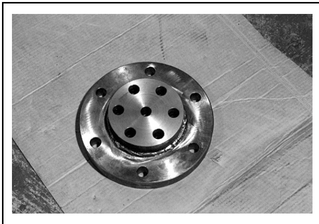
FIGURE 5 (MSSM0275AE) Shaft Cap Fixture Showing Raised Surface
