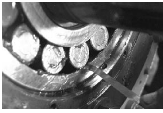
FIGURE 21 (MSSMA430AE) Determining Internal Radial Clearance
