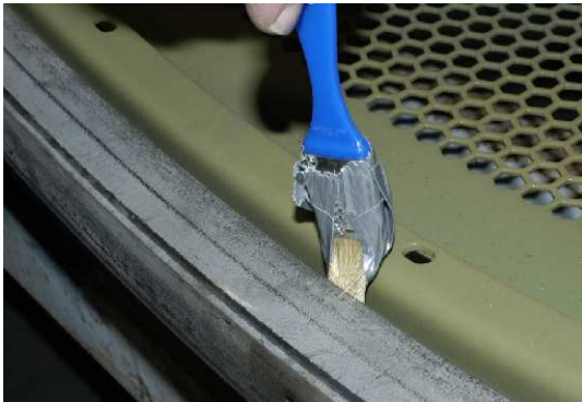
Figure 3: Adhesive applicator—1" paint brush, bristles held at an angle with tape
