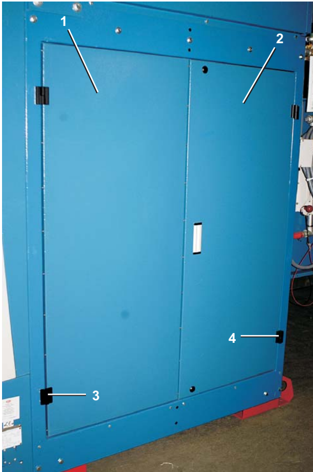
Side Doors used on Dryers since 2014
