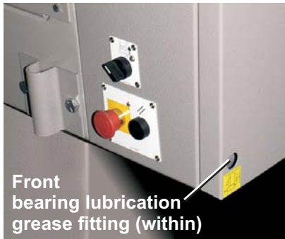
Figure 7: Shaft bearing lubrication lines
