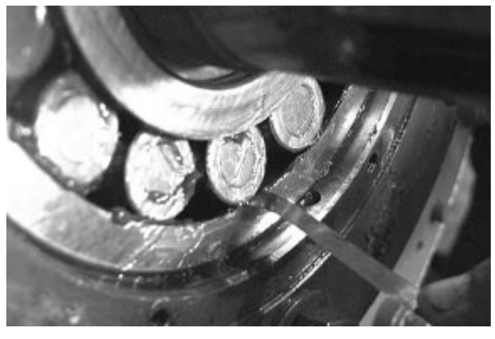
FIGURE 21 (MSSMA430AE) Determining Internal Radial Clearance
