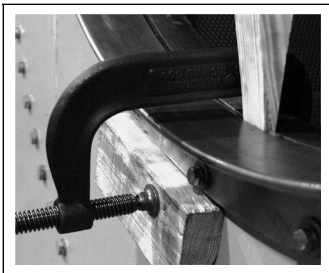
FIGURE 2 (MSSM0275AE) Clamping the Cylinder to the Shell Front
