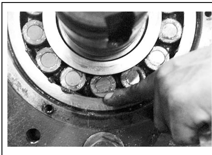
FIGURE 20 (MSSMA430AE) Where to Measure Internal Radial Clearance
