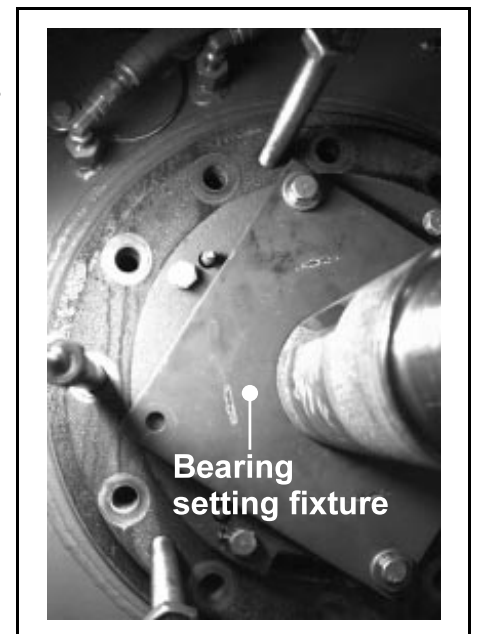
FIGURE 16 (MSSMA230AE) Bearing Setting Fixture
