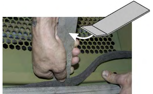
Figure 4: Seal installation tool—2" x 8" (5 x 20 cm) x 12 gauge steel plate, bent up on one end
