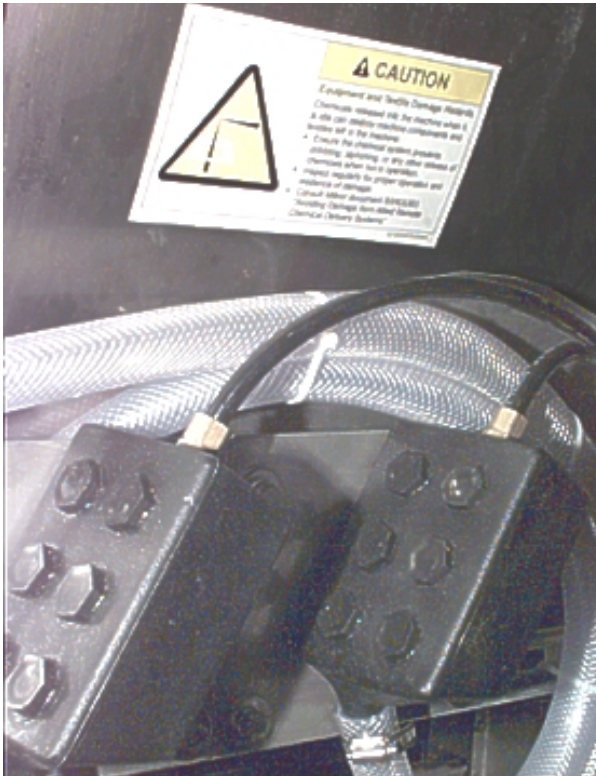
Figure 1: Pumped Chemical Inlets on CBW Batch Washer
