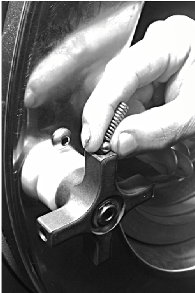
Figure 10: Inserting Ball and Spring in Handle Spoke
