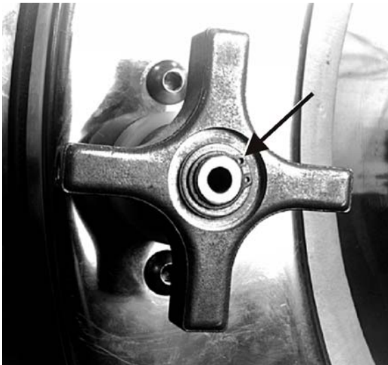
Figure 3: Front Retaining Clip and Thrust Washer
