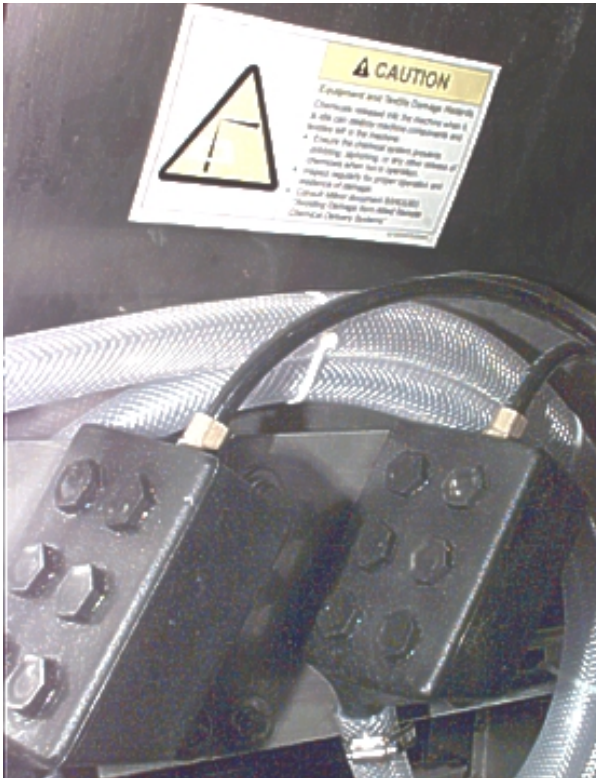
Figure 1: Pumped Chemical Inlets on CBW Batch Washer
