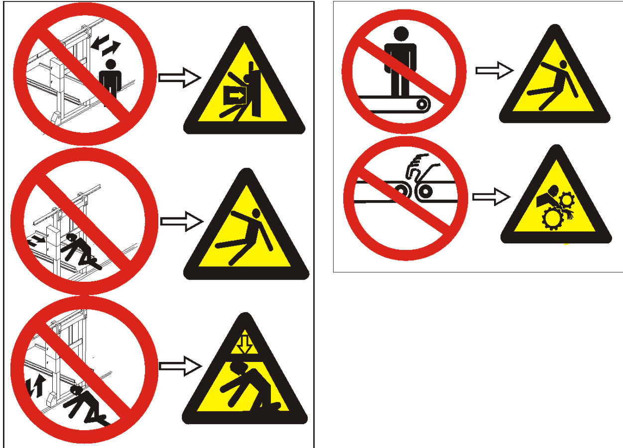
Figure 1: External Mechanical Hazards
