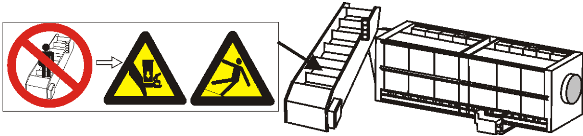
Figure 1: External Mechanical Hazards
