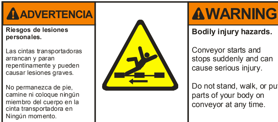
Figure 4: External Mechanical Hazards—Conveyor Starting and Stopping
