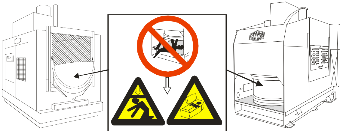
Figure 2: External Mechanical Hazards
