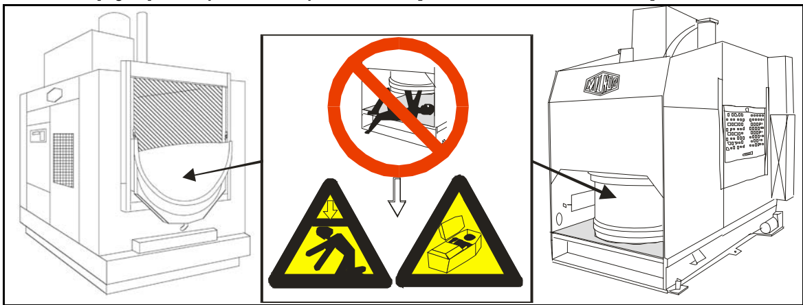
Illustration [Figure] 2: Risques mécaniques externes [External Mechanical Hazards]
