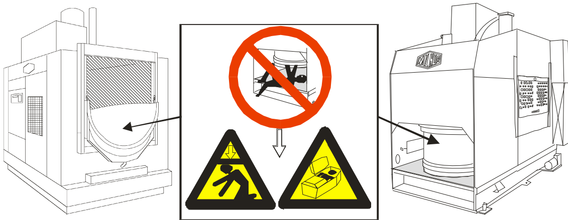
Figure 2: External Mechanical Hazards
