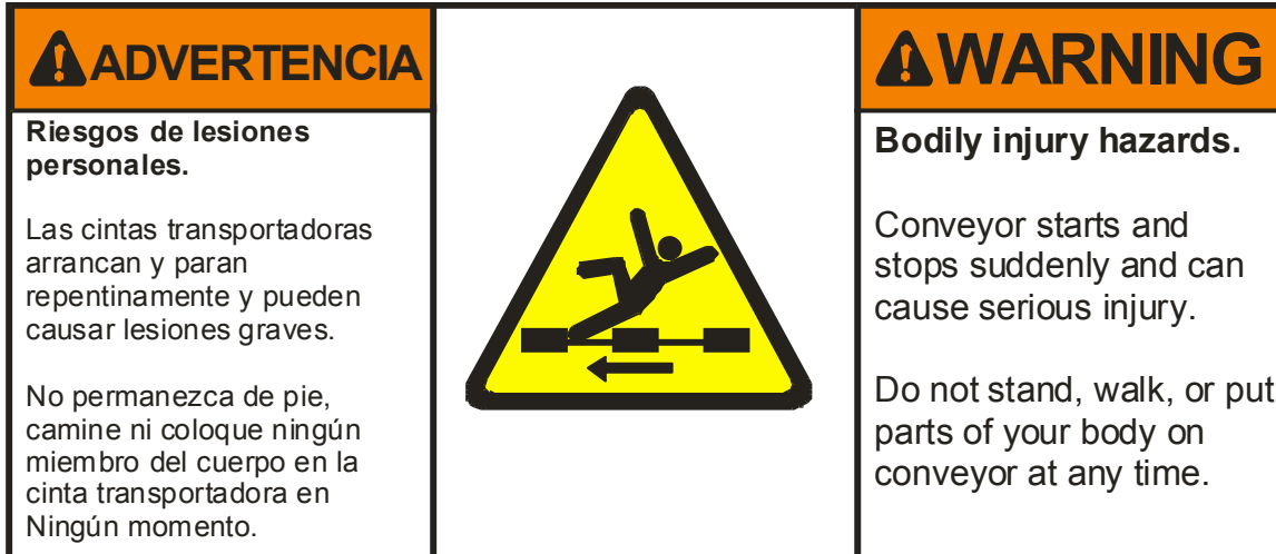
Figure 5: External Mechanical Hazards—Conveyor Starting and Stopping
