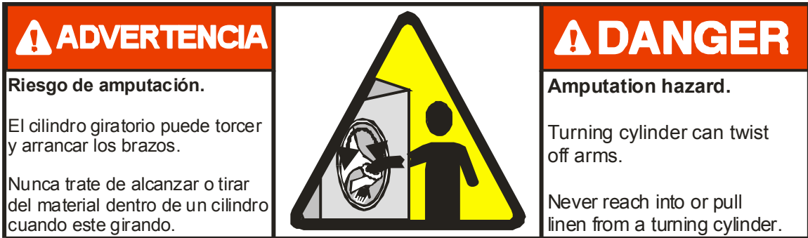
Figure 4: Cylinder and Processing Hazards—Grasping Goods in the Machine
