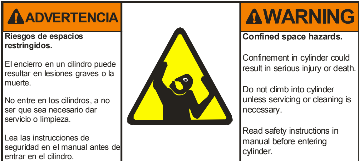
Figure 5: Cylinder and Processing Hazards—Confined Space
