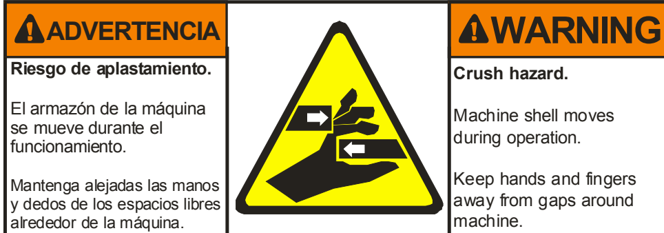
Figure 4: External Mechanical Hazards—Closing Gaps On Machine
