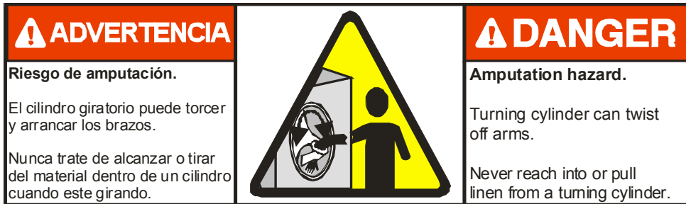
Figure 5: Cylinder and Processing Hazards—Grasping Goods in the Machine
