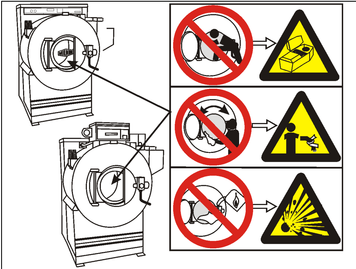
Figure 4. Cylinder and Processing Hazards
