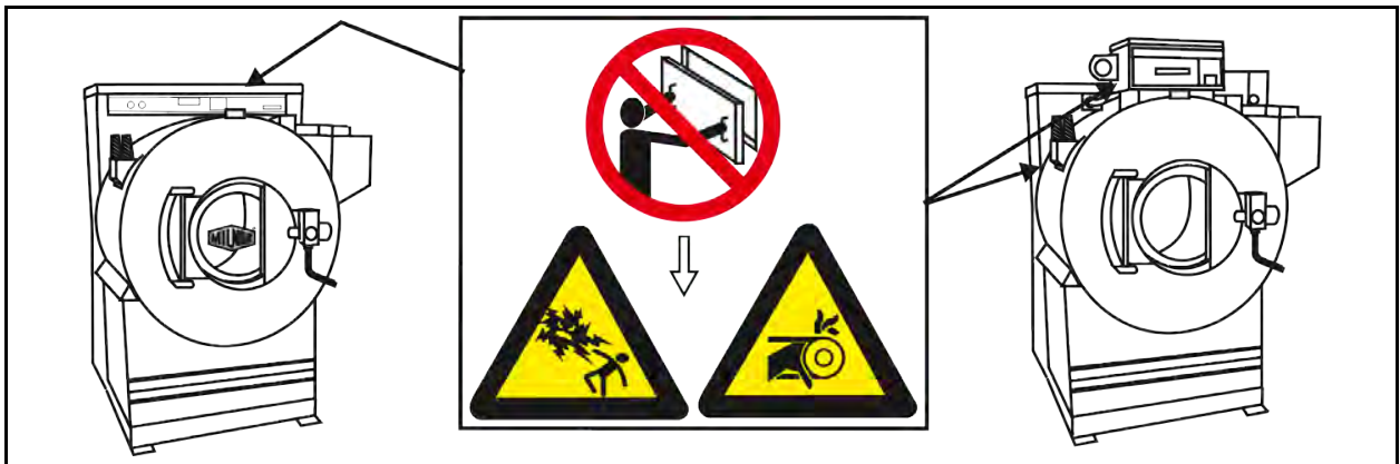
Figure 2. Internal Electrical and Mechanical Hazards
