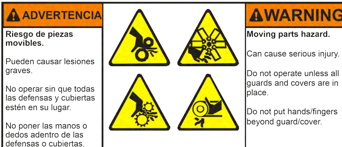
Figure 2. Internal Electrical and Mechanical Hazards—Moving Parts Behind Guards and Covers
