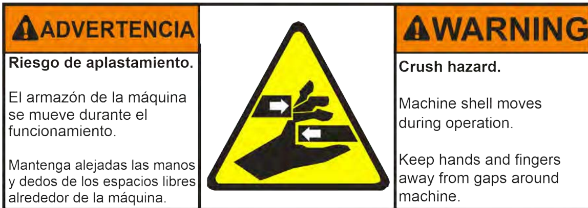
Figure 5. External Mechanical Hazards—Movement Around Machine
