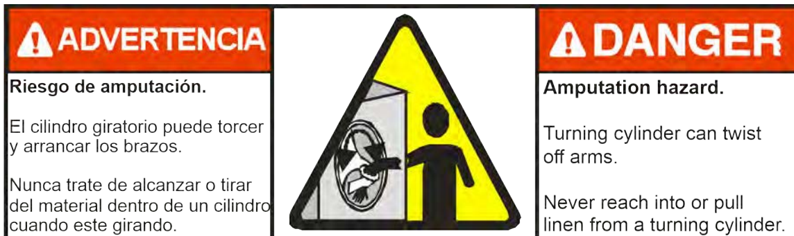
Figure 8. Cylinder and Processing Hazards—Grasping Goods in the Machine
