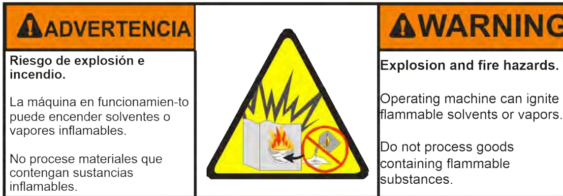
Figure 12. Cylinder and Processing Hazards—Explosives / Flammable Materials in Washer
