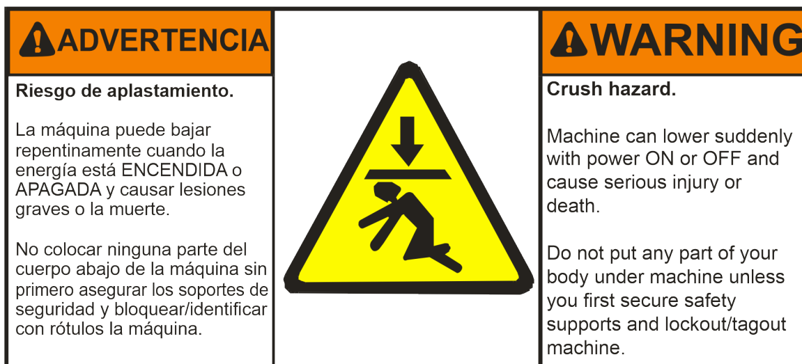
Figure 2. Internal Electrical and Mechanical Hazards—Descending Machine
