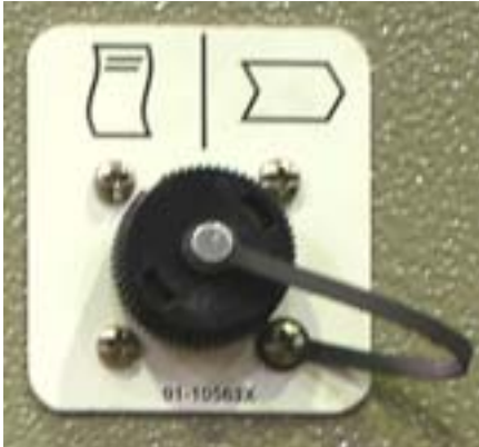
Figure 2: Serial Connection for Data Transfer
