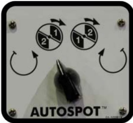
Figure 8: Autospot selector switch
